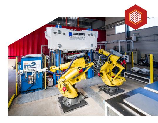
With Compression Resin Transfer Molding process, the resin mixture is fed into the mold when it is slightly open allowing partial impregnation. Then a compression stroke presses the resin through the preform for complete impregnation. By this way, an high-pressure resin injection allows the use of fast-curing systems.
